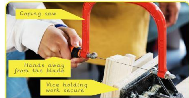
Remember to fix or hold your wood securely on the bench hook or vice when sawing, and keep your fingers out of the way of the blade.
